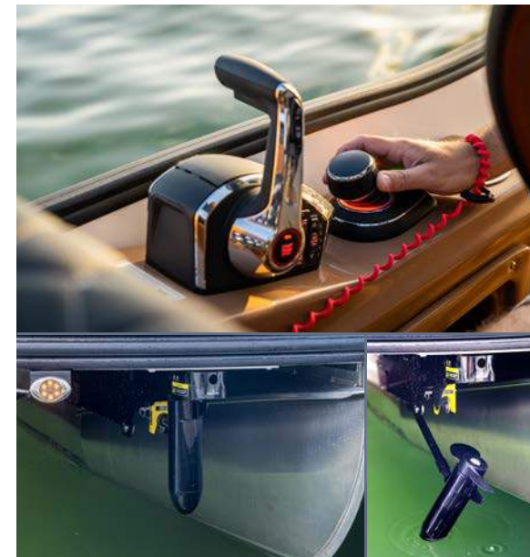
SINGLE-ENGINE JOYSTICK PILOTING (Available on Solstice, Grand Mariner and Crowne models)
